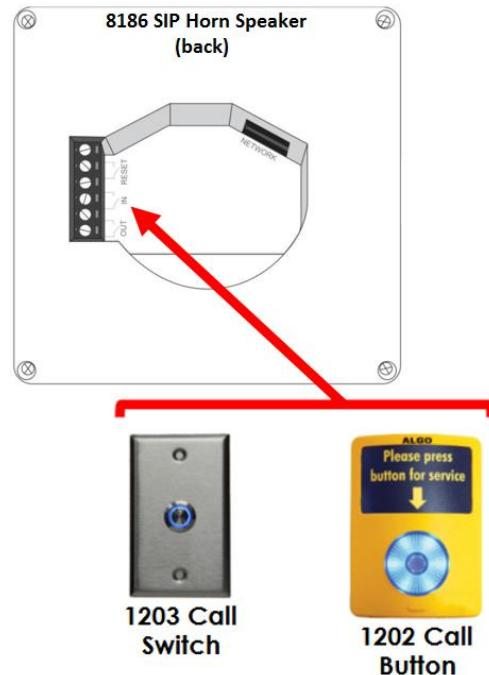
**1202 Call Button:** A pair of wires from the terminal block on the back of the 8186 SIP Horn Speaker can connect to the **centre pair** of the modular connector at the back of the Call Button.
