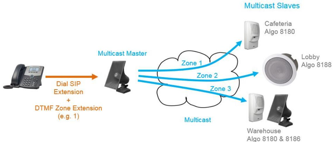
Alternatively, multiple SIP extensions can be registered on the master device. Each extension is mapped to a unique zone, allowing zones to be called directly (for instance from speed-dial keys) without the use of DTMF. See "Additional Features > More Page Extensions".
