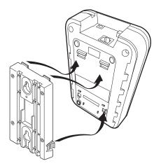
Figure 10: Attach Wall Mount Stand to Base Unit
