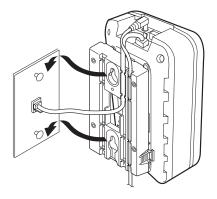
Figure 7: Mount Base Unit on Wall Plate
