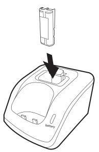
Figure 23: Charge Spare Battery
