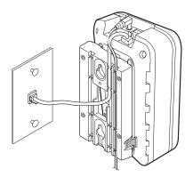
6 Place the base unit on the posts of the wall plate and pull down until the base unit is firmly seated.
