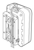
6 Place the base unit on the posts of the wall screws and pull down until the base unit is firmly seated.
