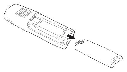
Figure 19: Remove Battery Cover
