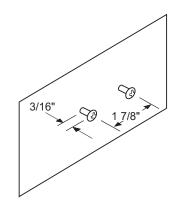
Figure 17: Insert Mounting Screws into Wall
