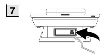
Connect the analog adjunct such as a modem, fax machine, or analog telephone to the module.
