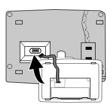
Carefully align the module ribbon cable to the mating receptacle on the bottom of the telephone and insert slowly.
