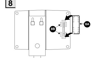
The desktop stand has slots in which you can store the cover ( ) you removed from the module opening (see Step 2) in case you need to reinsert the cover at a later time.
