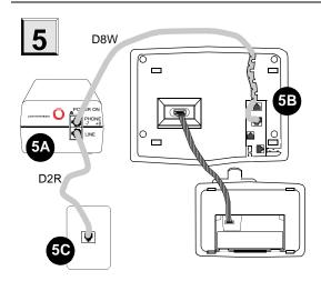
Connect the stand-alone local auxiliary power supply (๑). With the D8W cord, connect the auxiliary power supply (the PHONE jack) to the Line jack on the telephone (๑). Then, connect the power supply (the LINE jack on the power supply) to a wall jack (๑).
