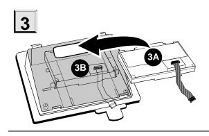
Install the module (3A) in the desktop stand (3B). Push down until you hear the module snap in place.
