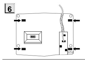
Replace the stand and module by lowering the desktop stand onto the bottom of the telephone. The tabs on the stand must snap into the appropriate slots on the bottom of the telephone. (These slots are marked with arrows in the accompanying drawing on the left.)
