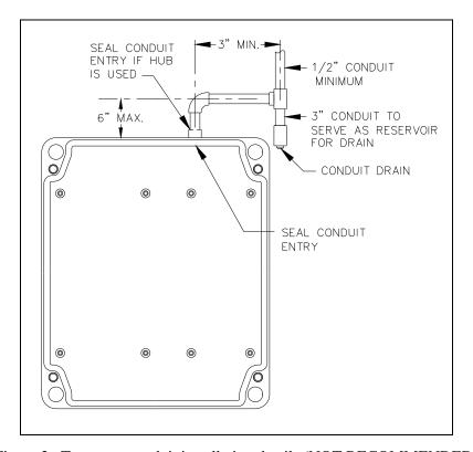
Figure 2. Top entry conduit installation details (NOT RECOMMENDED)
