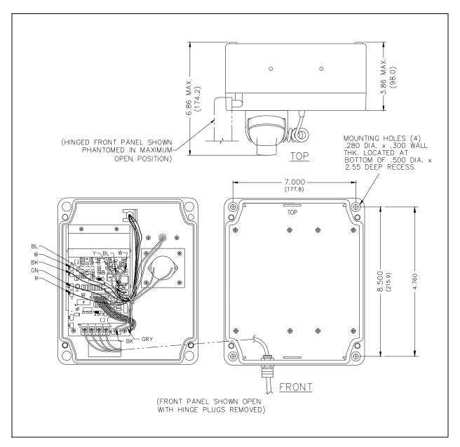
Figure 8. Model 246-001 Mounting Diagram
