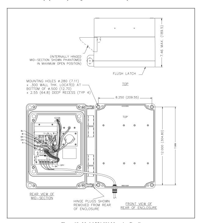
Figure 10. Model 256-001 Mounting Detail
