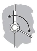
**CAUTION** To avoid breaking the boom, only rotate it up and over 180°.
