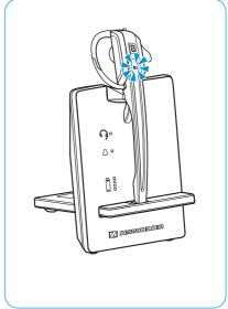
▶ Place the headset into the magnetic holder of the base station. The Headset LED lights up blue and the rechargeable battery is being charged. The Charge status LED on the base station indicates the charge status:
