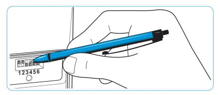
Configuring the handset lifter/hook switch – DIP switches 1 and 2
